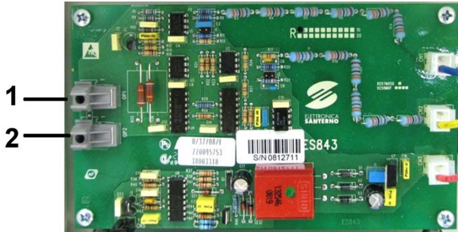
Figure 37: ES843 Bus-bar Voltage Acquisition Board
