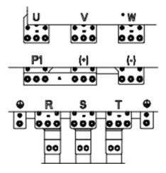
Figure 4-17 Main circuit terminals for the 0400- 1000 models
