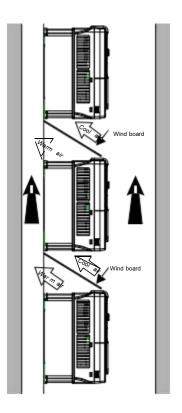
Figure 4-4 Vertical installation
