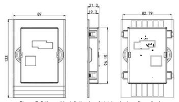
Figure B-2 Keypad Installation bracket (standard configuration)
