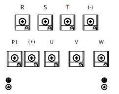
Figure 4- 14 Main circuit terminals for the 0160 – 0185 models
