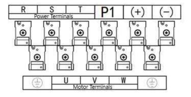
Figure 4- 16 Main circuit terminals for the 0250 – 0355 models
