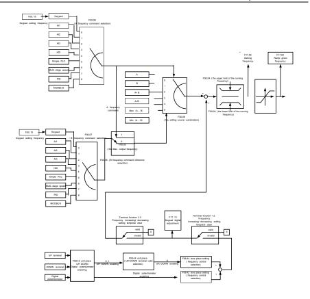
SG200 series VFDs support the shifting between different reference channels and the detailed shifting rules is as below:
