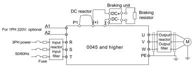
Figure 4-8 Main circuit wiring diagram for the 0045 and higher models
