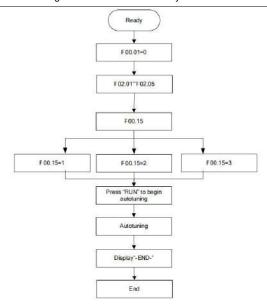
The control performance of the VFD is based on the established accurate motor model. The user has to carry out the motor auto-tune before first running (take motor 1 as the example).
