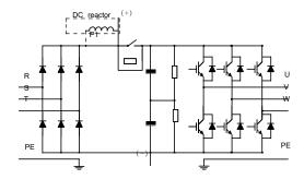
Figure 3-2 Main circuit diagram (for the 0045 and higher models)
