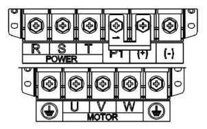
Figure 4- 13 Main circuit terminals for the 0090 – 0132 models
