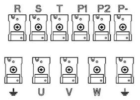
Figure 4- 15 Main circuit terminals for the 0200 - 0250 models
