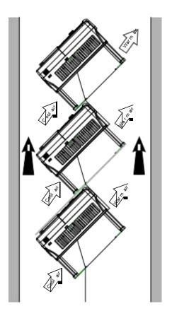
Figure 4-5 Tilt installation
