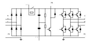
Figure 3-1 Main circuit diagram (for the 0037 and lower models)
