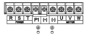
Figure 4- 12 Main circuit terminals for the 0045 -0075 models
