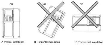
Figure 4-1 Installation direction of the VFD
