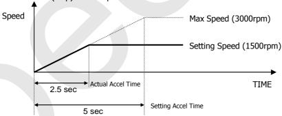
**Setting example 2** If FUN\_33 is set to 'Ref Speed' and speed command and acceleration time is set to 500rpm and 1500rpm for 5 seconds, respectively, it takes 5 seconds to accelerate from the standstill to 1500rpm.
