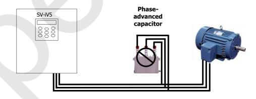
③ Cable between inverter output and motor should be less than 300m long. If cable gets long, surge voltage appears across motor terminals depending on the cable parameters. Especially, in 400V class motor case, insulation withstanding voltage may be decreased. Use an insulation-reinforced motor or surge reduction filter when 400V class motor is used.
