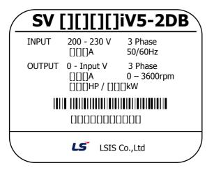
Inverter Model Name Input Power Source Specifications Rated Capacity **Output Power Source Specifications** Running Freq. / Rated Output Current **Output Capacity** Bar Code Serial Code
