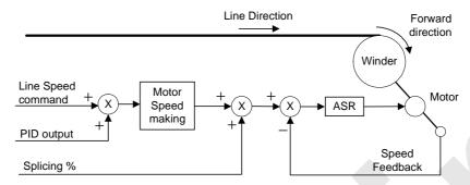
Figure 1. Roll Rotating Direction at the time of Rewind/Overwind Setting, Forward Direction Operation Command
