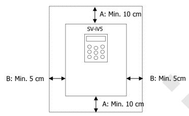
At least the room that 30 cm from upper and lower of inverter and 20 cm from left and right of inverter is required for installing more than 30 kW products.
