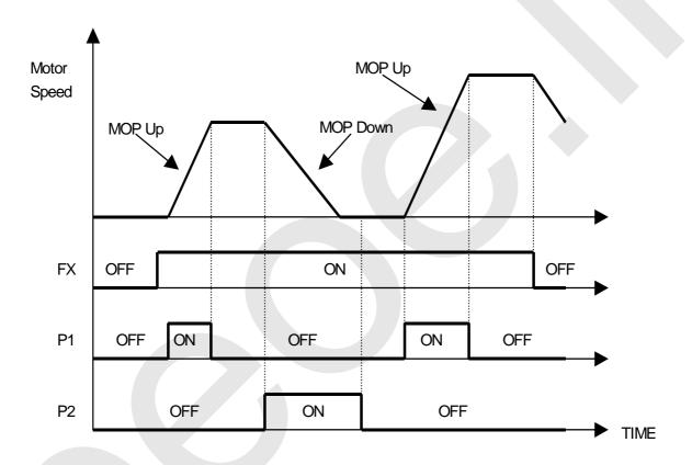
(MOP Save example 2) In case terminal input assigned to MOP Save function is ON, operation speed at that instant is memorized and operates at the saved speed when operation resumes.
