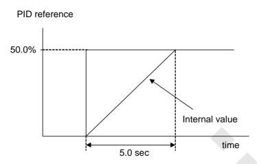
Tension Command where Ramp Time is applied
