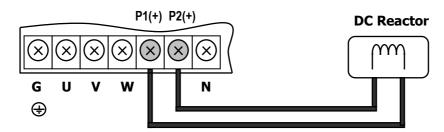
3.3.6 Wiring DB Unit (Option) (AC power input: 30kW and higher)
