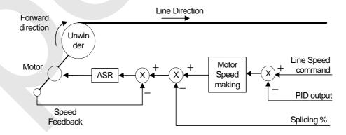
Figure 3. Roll Rotating Direction at the time of Unwind/Overwind Setting, Forward Direction Operation Command
