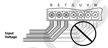
② Never connect the phase advancing capacitor to the inverter output. If already installed, remove the phase-advanced capacitor clearly.
