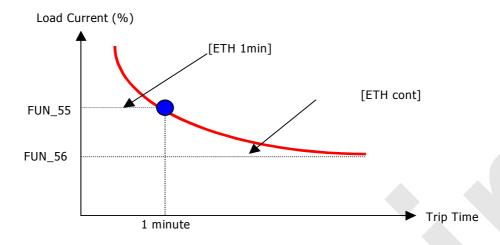
[Motor i2t Characteristic Curve]
