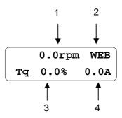
The status of the screen as above is called "Home Screen of Display Group" or "Home Screen", and you can return to this home screen by pressing SHIFT/ESC key. Each item on the screen shows the associated information as shown in the table below.
