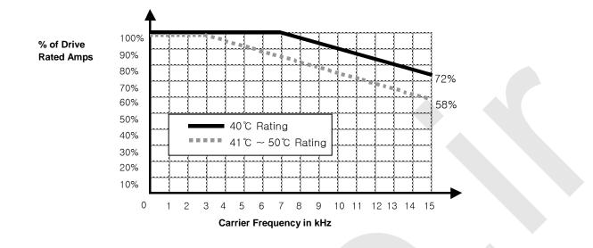
Load and ambient temperature classified by the Carrier Frequency
