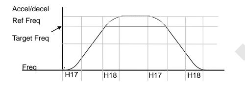
If Target Frequency is below Max Frequency, the waveform will be shown with the top portion cut out.
