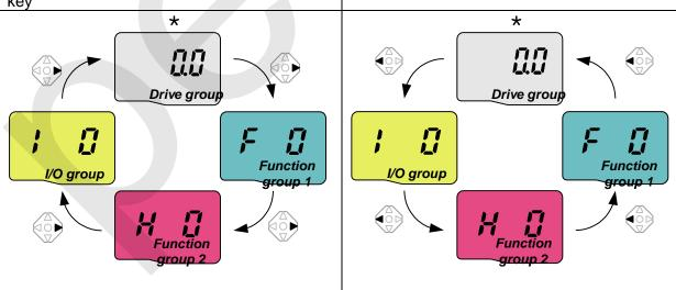
\* Target frequency can be set at **0.0** (the 1<sup>st</sup> code of drive group). Even though the preset value is 0.0, it is user-settable. The changed frequency will be displayed after it is changed.
