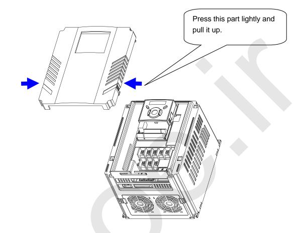
• To change the inverter fan: Press the both sides of bottom cover lightly and pull out to your side.
