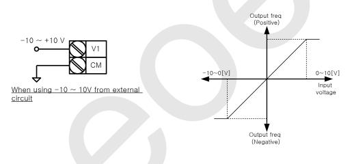
I 2 ~ I 5: Setting input range and corresponding frequency to -10V ~ 0V V1 input voltage
