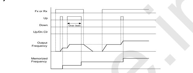
When F65 is 2: It is increased as many as step frequency set as F66 at the rising edge of multifunction input set as UP and if it is activated for 3 second, it operates like something set as "0". It is decreased as many as step frequency set as F66 at the rising edge of multi-function input set as DOWN and if it is activated for 3 second, it operates like something set as "0" and the accel/decel time is same with when stetted as "0".
